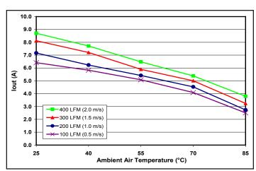
Figure 3: Thermal Derating (max output currnet vs. ambient air temperature) for encased converter without heatsink, at airflow rates of 100 LFM through 400 LFM. Air flows across the converter from input to output (nominal input voltage).
