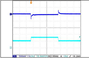
Figure 5: Output Voltage Response to Step-Change in Load Current (50%-75%-50% of Iout(max);  $dI/dt = 0.1A/\mu s$ . Load cap:  $15\mu F$  tantalum cap and  $1\mu F$  ceramic cap. Ch 1: Vout, Ch 2: Iout (20 Iout).
