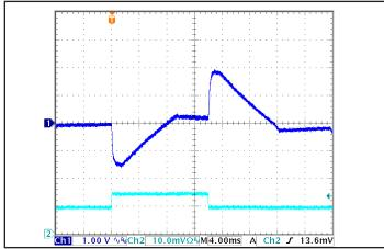
Figure 5: Output Voltage Response to Step-Change in Load Current (50%-75%-50% of Iout(max);  $dI/dt = 0.1A/\mu s$ . Load cap:  $100\mu F$  electrolytic cap and  $1\mu F$  ceramic cap. Ch 1: Vout, Ch 2: Iout (5 Iout).
