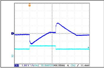
Figure 5: Output Voltage Response to Step-Change in Load Current (50%-75%-50% of Iout(max); dI/dt = 0.1A/\mus. Load cap: 100\muF electrolytic cap and 1\muF ceramic cap. Ch 1: Vout, Ch 2: Iout (10 A/div).
