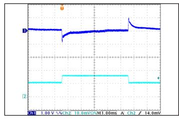
Figure 5: Output Voltage Response to Step-Change in Load Current (50%-75%-50% of Iout(max);  $dI/dt = 0.1A/\mu s$ . Load cap:  $1\mu F$  ceramic cap. Ch 1: Vout, Ch 2: Iout (10 A/div).
