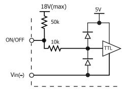
Figure B: Internal ON/OFF Pin Circuitry
