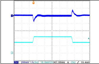
Figure 5: Output Voltage Response to Step-Change in Load Current (50%-75%-50% of Iout(max);  $dI/dt = 0.2A/\mu s$ ). Load cap:  $15\mu F$  tantalum cap and  $1\mu F$ ceramic cap. Ch 1: Vout, Ch 2: Iout (20A/div).
